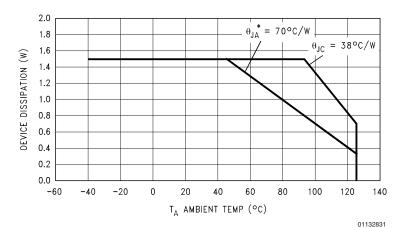
$^{\star}\theta_{JA}$  = Thermal Resistance with 2 square inches of 1 ounce Copper tied to Pins 1, 8, 9 and 16.
