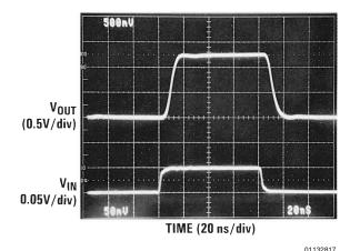
FIGURE 4. Reducing R<sub>f</sub> for Large Closed Loop Gains, R<sub>f</sub> =  $500\Omega$
