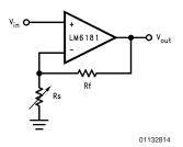
FIGURE 2. R<sub>S</sub> Is Adjusted to Obtain the Desired Closed Loop Gain, A<sub>VCL</sub>
