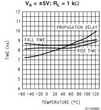
SMALL SIGNAL PULSE RESPONSE vs TEMP,
