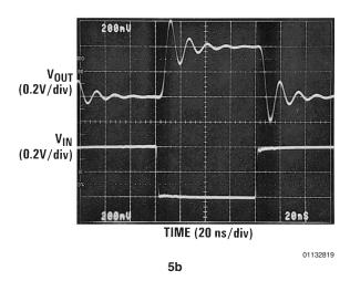
FIGURE 5.  $A_V = -1$ , LM6181 Can Directly Drive 50 pF of Load Capacitance with 70 ns of Ringing Resulting in Pulse Response
