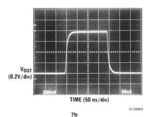
FIGURE 7. RC Limits Amplifier Bandwidth to 50 MHz, Eliminating Peaking in the Resulting Pulse Response
