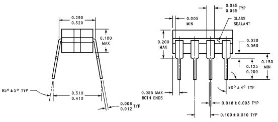
8-Pin Ceramic Dual-In-Line Package Order Number LM6181AMJ/883 **NS Package Number J08A**
