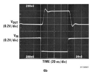
FIGURE 6. Resistive Isolation of  $C_L$  Provides Higher Fidelity Pulse Response.  $R_f$  and  $R_S$  Could Be Increased to Maintain  $A_V = -1$  and Improve Pulse Response Characteristics.
