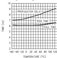
SMALL SIGNAL PULSE RESPONSE vs TEMP,
