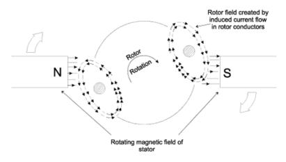
Reliance Electric's diagram of movement within an electromagnetic motor.
