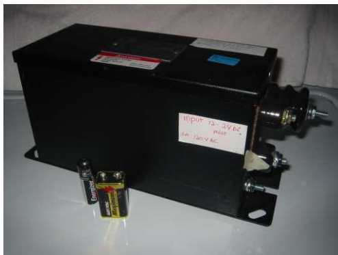
15,000 v Neon Transformer
